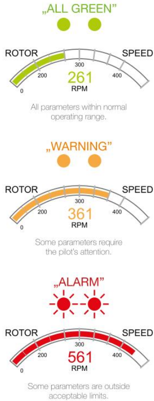
Fig. 7. The idea of flight parameter status information
